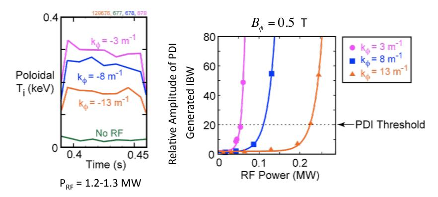
Predicted power threshold is consistent with previous reflectometer measurements (100 to 300kW), (Wilgen 2005).
